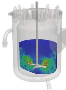
Figure 1. CFD Simulation: Visual of fluid shear stress on 2L lab reactor at 300RPM using P4 type impeller
